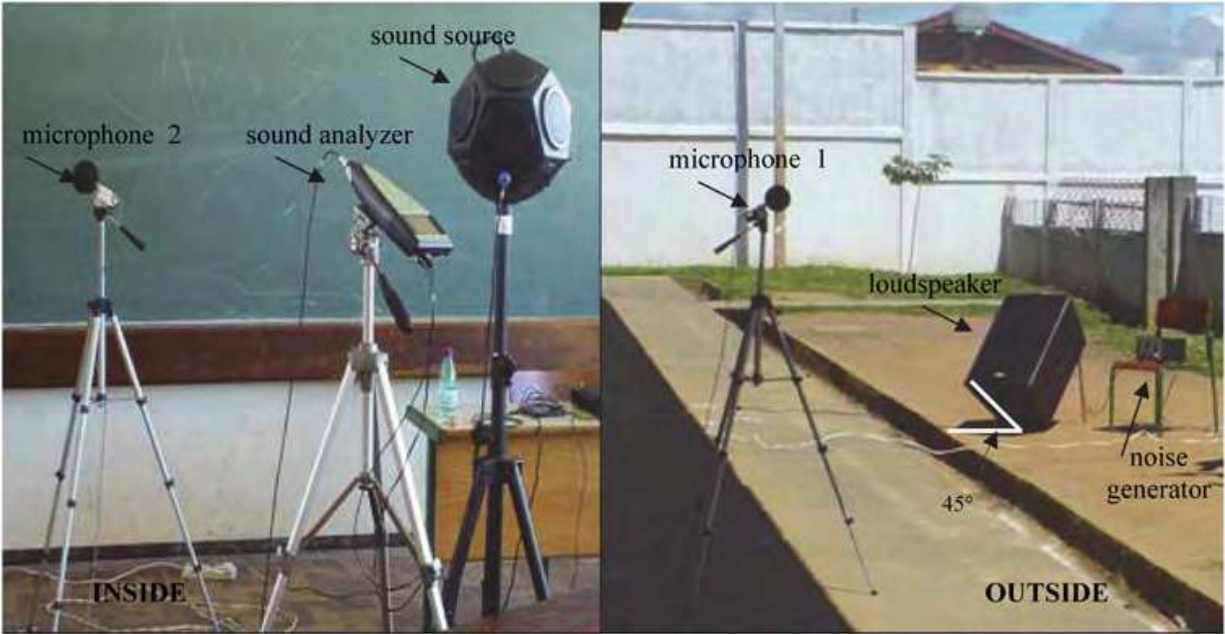
Fig. 2. Measurement of façade insulation according to ISO 140-5 10
