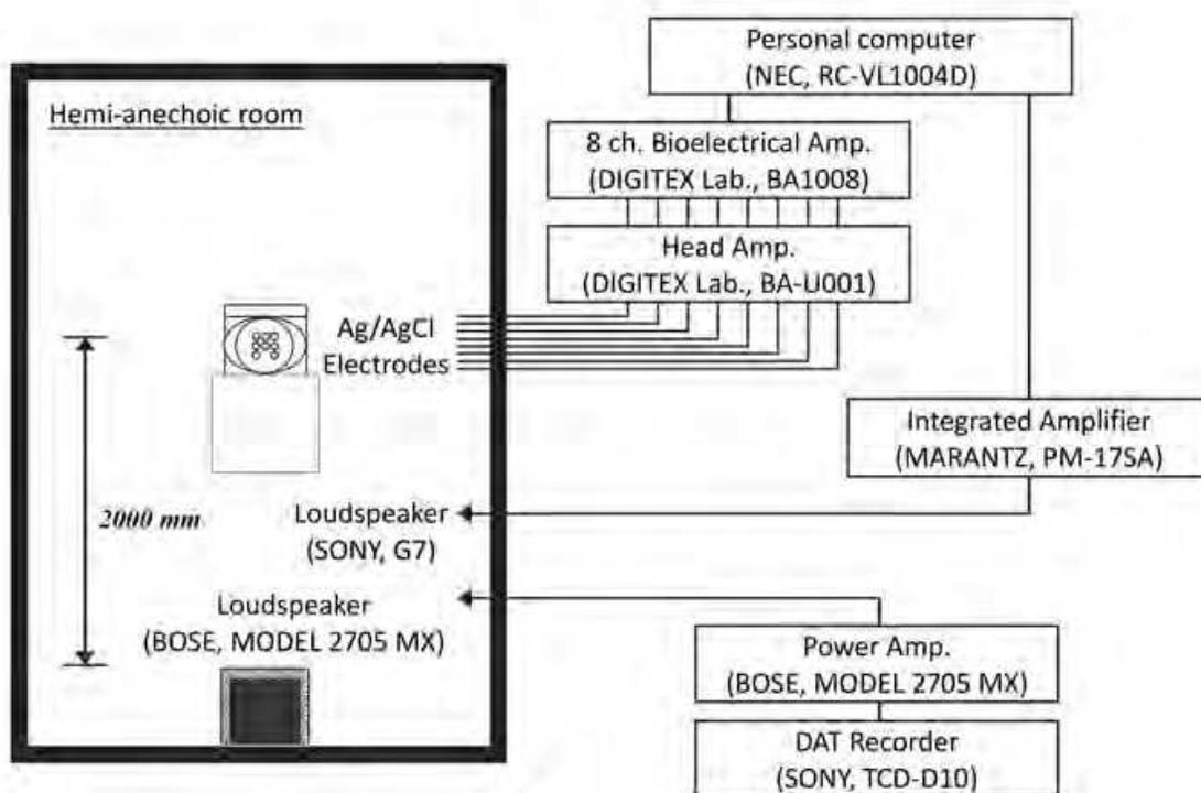
Fig. 2. Block diagram of experimental system
