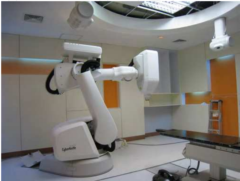
Fig. 12. CyberKnife Robotic Radiosurgery system
