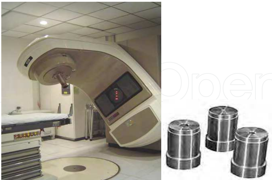
Fig. 11. Linac-based radiosurgery machine and circular collimators
