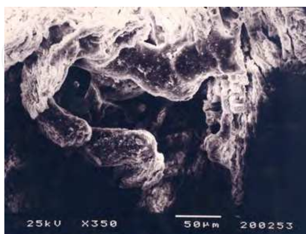
Fig. 8. Enamel. 800 mj. 5 Hz. Without water cooling. Melted and resolidified enamel. This texture is highly acid resistant.
