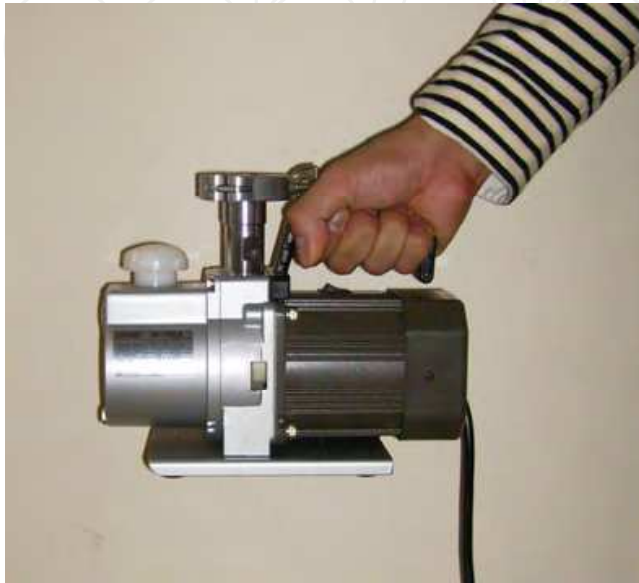
Fig. 5. A small rotary vacuum pump.
