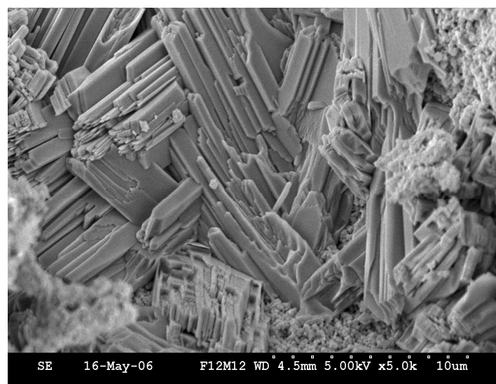
Fig. 10. View represents the microstructure of the Feral treated with 12 M NaOH solutions and cured at 12 h.
