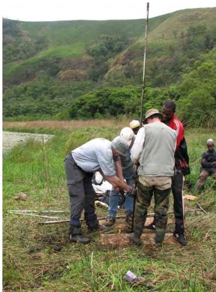
Fig. 4. Coring on Lake Bambili using the Russian manual corer.
