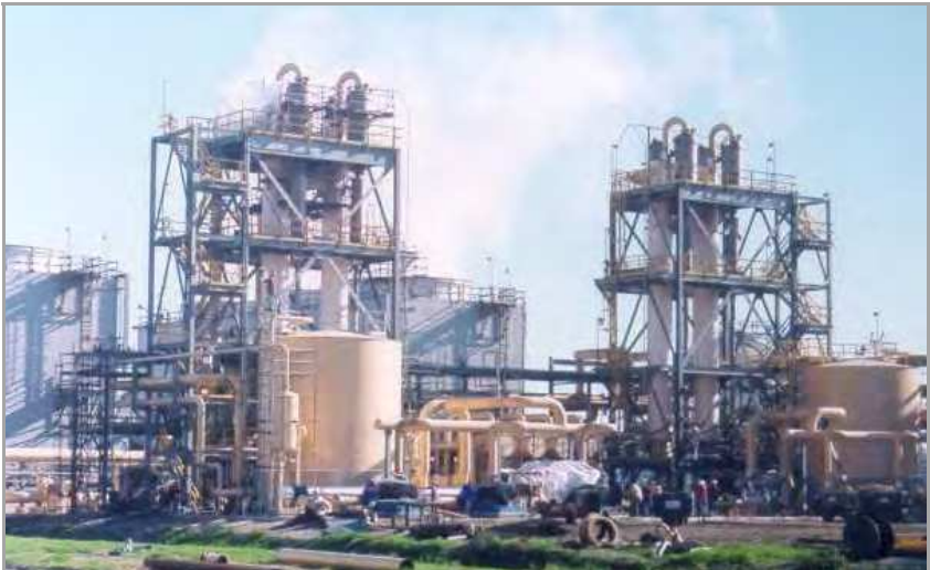
Fig. 14. Installation of 4 600 m 2 self-cleaning surface replacing 24 000 m 2 conventional surface.
