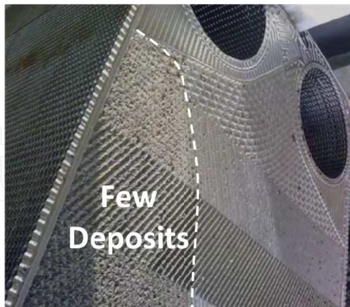
Fig. 8. Deposits formed on the surface of NT-plate.
