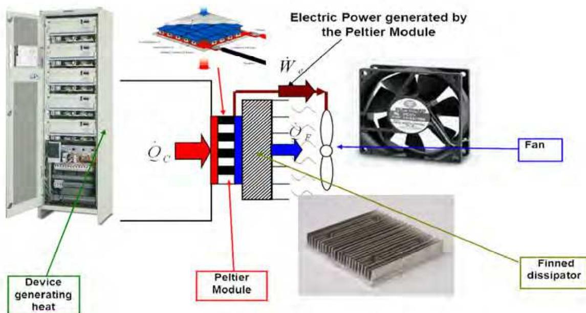
Fig. 12. Sketch of a thermoelectric self-cooling system.
