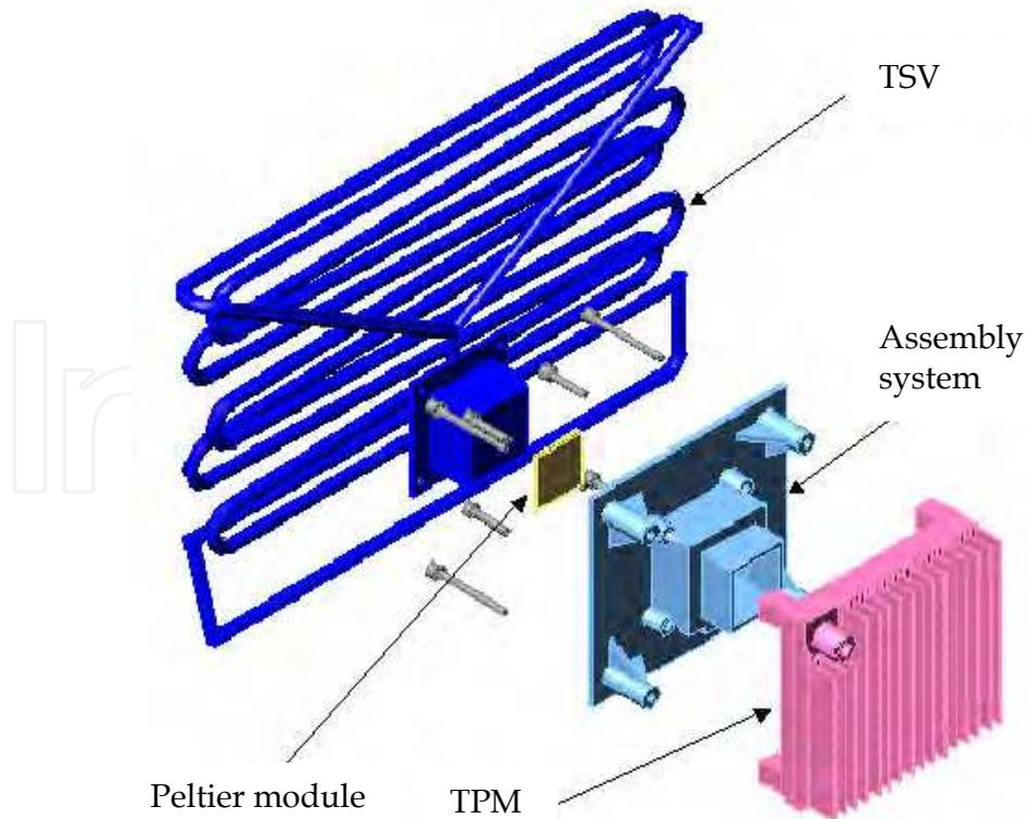
Fig. 10. Thermoelectric device with the heat exchangers TSV and TMP.
