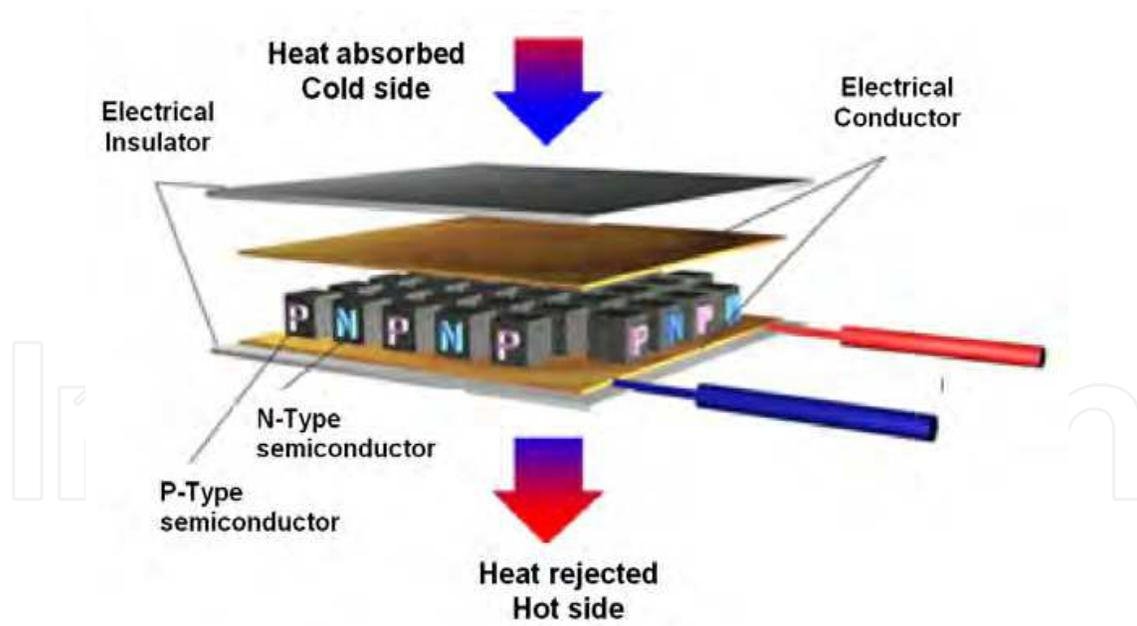
Fig. 1. Sketch of a Peltier module working as refrigerator.
