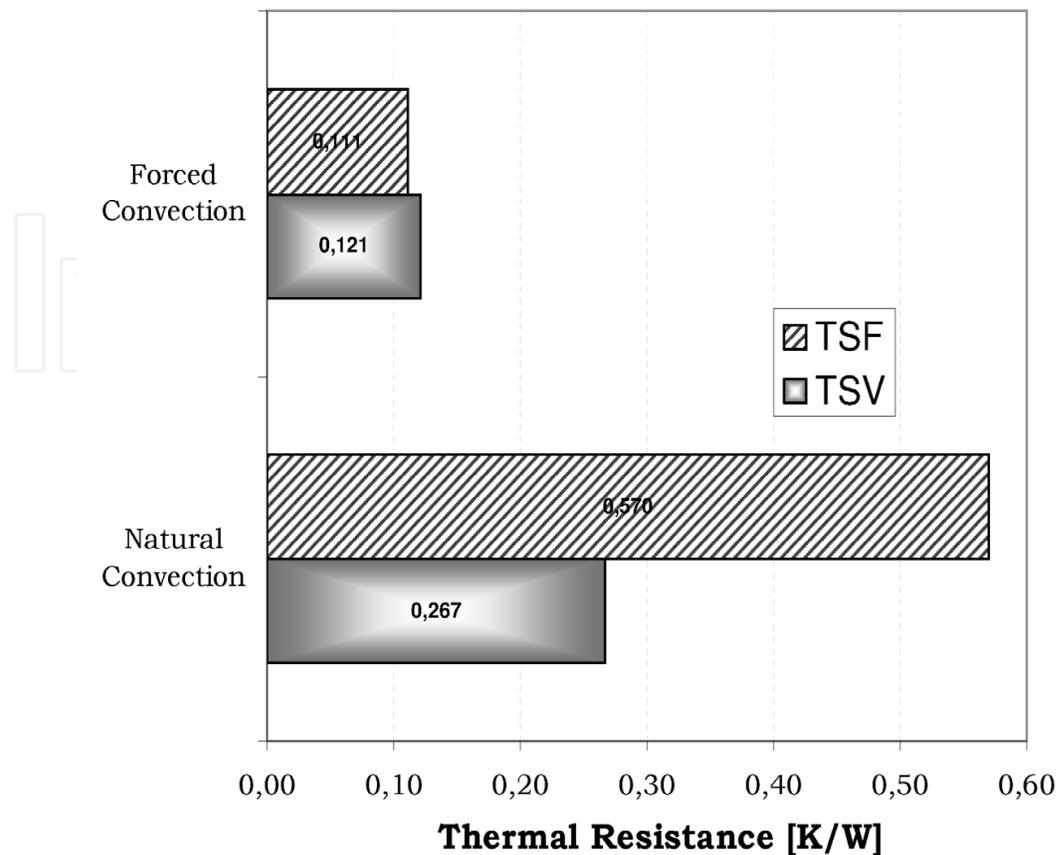
Fig. 8. Thermal resistances of TSF and TSV for natural and forced convection.
