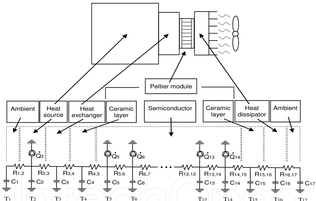
Fig. 3. Sketch and discretization of a thermoelectric generator.
