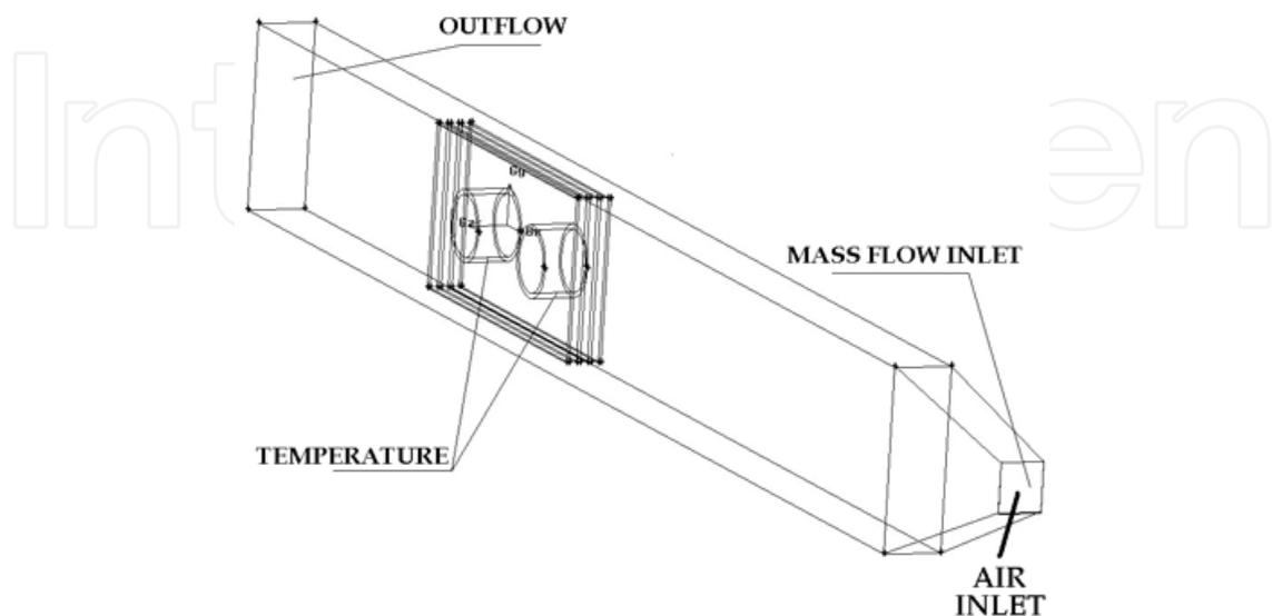
Fig. 15. Geometry of the numerical model of the test rig and boundary conditions types.
