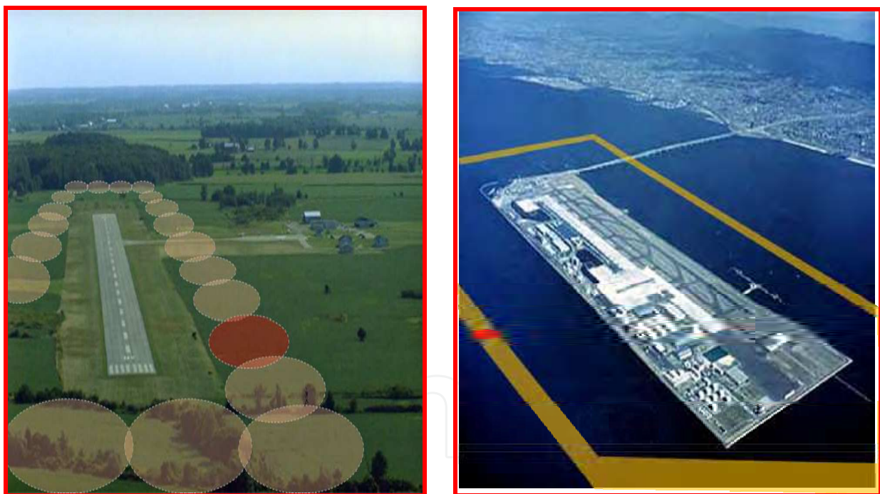
Fig. 9-10. The SFCO -sensor based Early Warning Security System can secure the runway and specific underwater perimeter with the invisible and totally passive security net, and can detect over the ground and underground, as well as underwater moving intruders.
