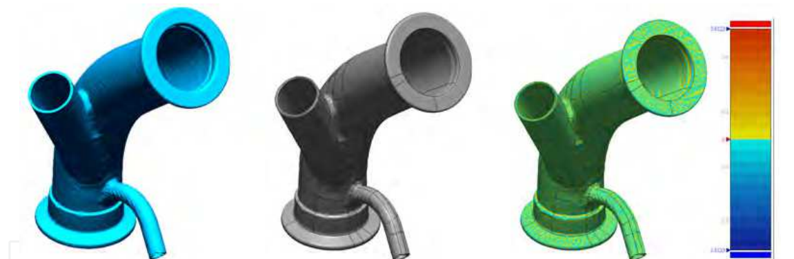
Fig. 14. Results of the tubing example tested using Rapidform , (a) polygon mesh (589,693 triangles), (b) NURB surface model (185 patches), and (c) deviation analysis
