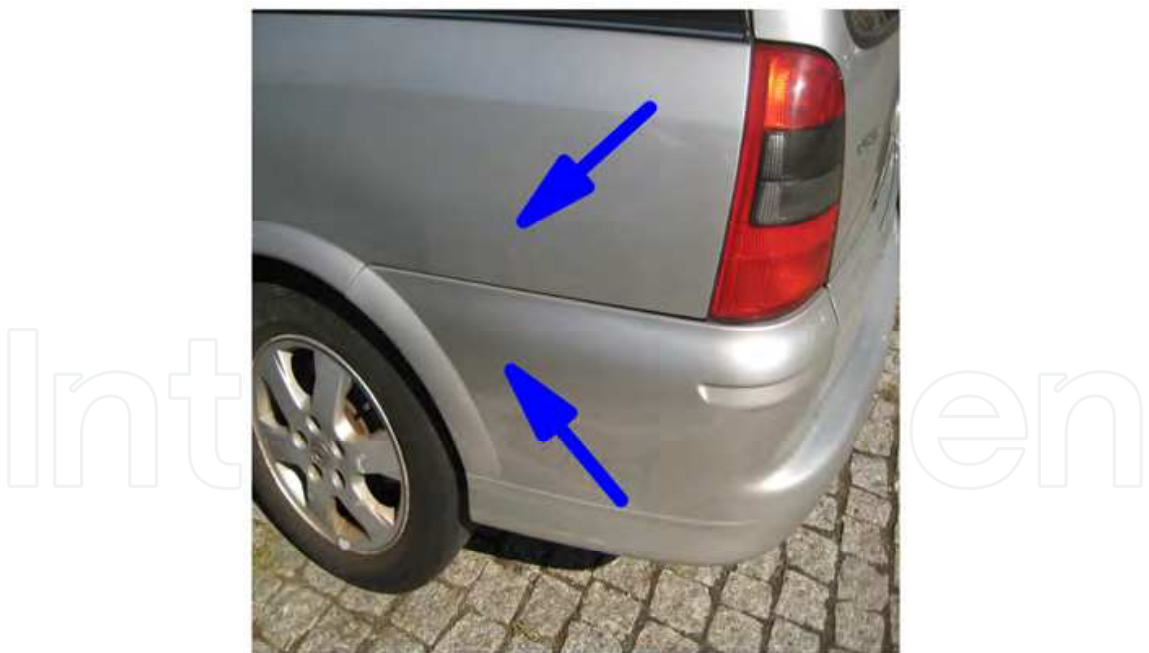
Fig. 3. Example of colour harmony in a silver-like coating containing aluminium flakes. Current colour designs must achieve no perceptible colour differences between the different external parts that integrate the car such as the car body and the fenders.
