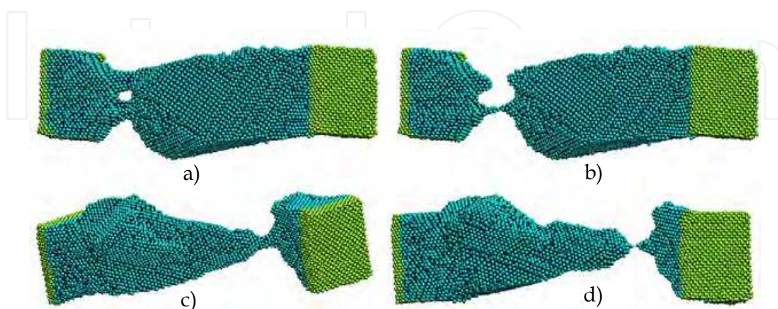
Fig. 18. (a) and (b) the formation of rupture of specimen with no defects for shear simulation, (c) and (d) that of specimen with scratching depths of 5a_0 .
