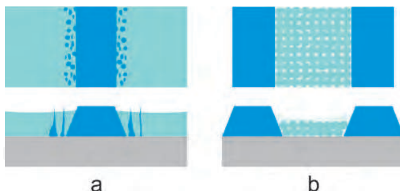
Fig. 14. Some variations of the interface morphology at the sub-micrometer scale that have been (left) or at the micrometer scale that could be (right) realized with self-aligned pattern transfer. Left: nanocolumnar structures of material A between the areas of bulk materials A and B, respectively. Right: gap between strips of material A filled with nanoparticles before the deposition of material B.
