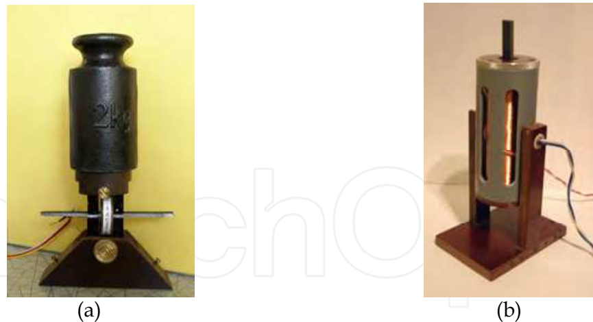
Fig. 9. The arrangements, used for the measurements. (a): The samples are magnetized by the short coil placed around middle of each sample and a pair of soft passive yokes closes the magnetic circuit from bottom and top. (The 2 kg weight is used only for pressing the yokes better on the sample surfaces.) (b): The samples are magnetized inside the long solenoid.
