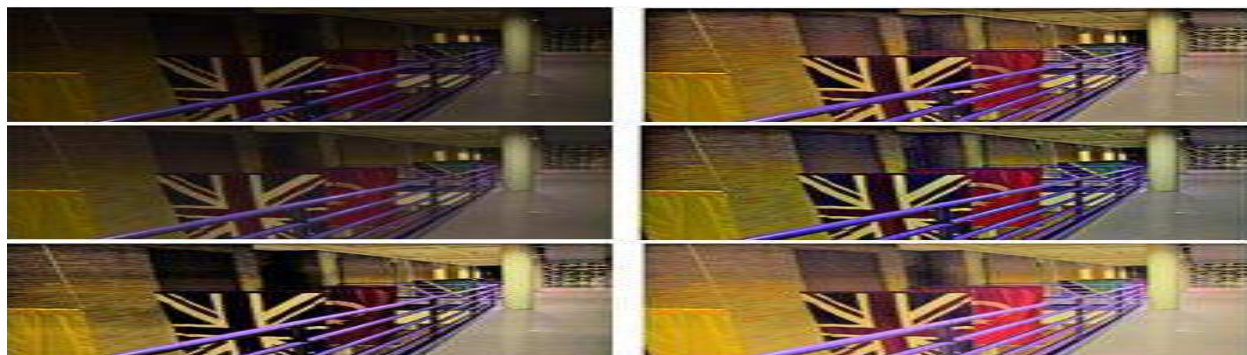
Fig. 2. Comparisons of Enhancement Techniques: (top-left) Original; (top-right) IRME; (middle-left) Gamma correction, g = 1.4 ; (middle-right) MSR; (bottom-left) AINDANE; (bottom-right) ETNUD.
