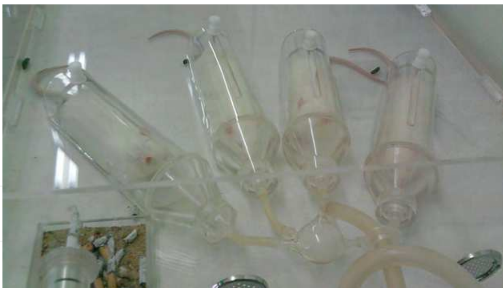
Fig. 1. Apparatus created by the team of the Laboratory of Genetics and Cell Therapy – GenTe Cel to induce emphysema by cigarette smoke.
