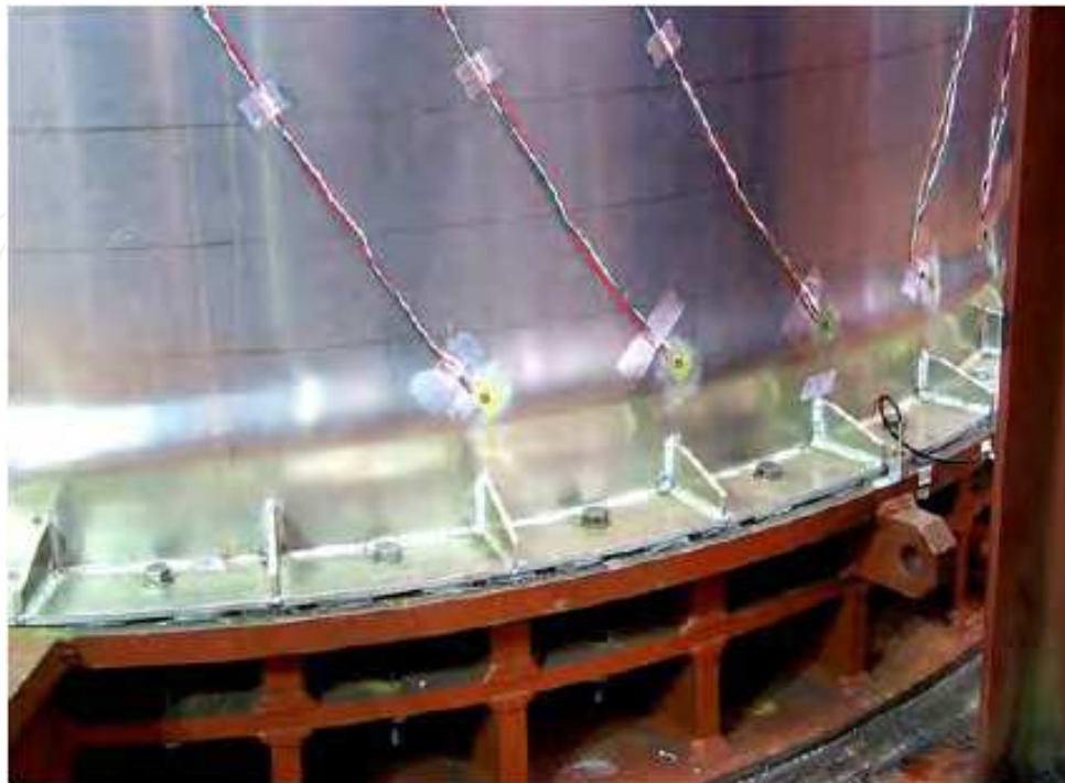
Fig. 3. Typical mode of elephant foot bulge. (Ito et al., 2003)
