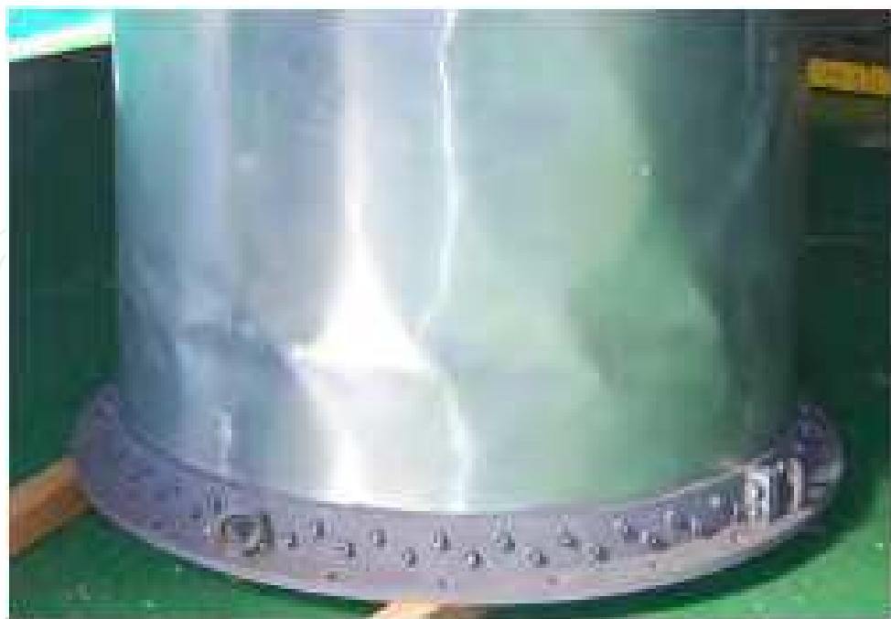
Fig. 2. Typical mode of diamond buckling.
