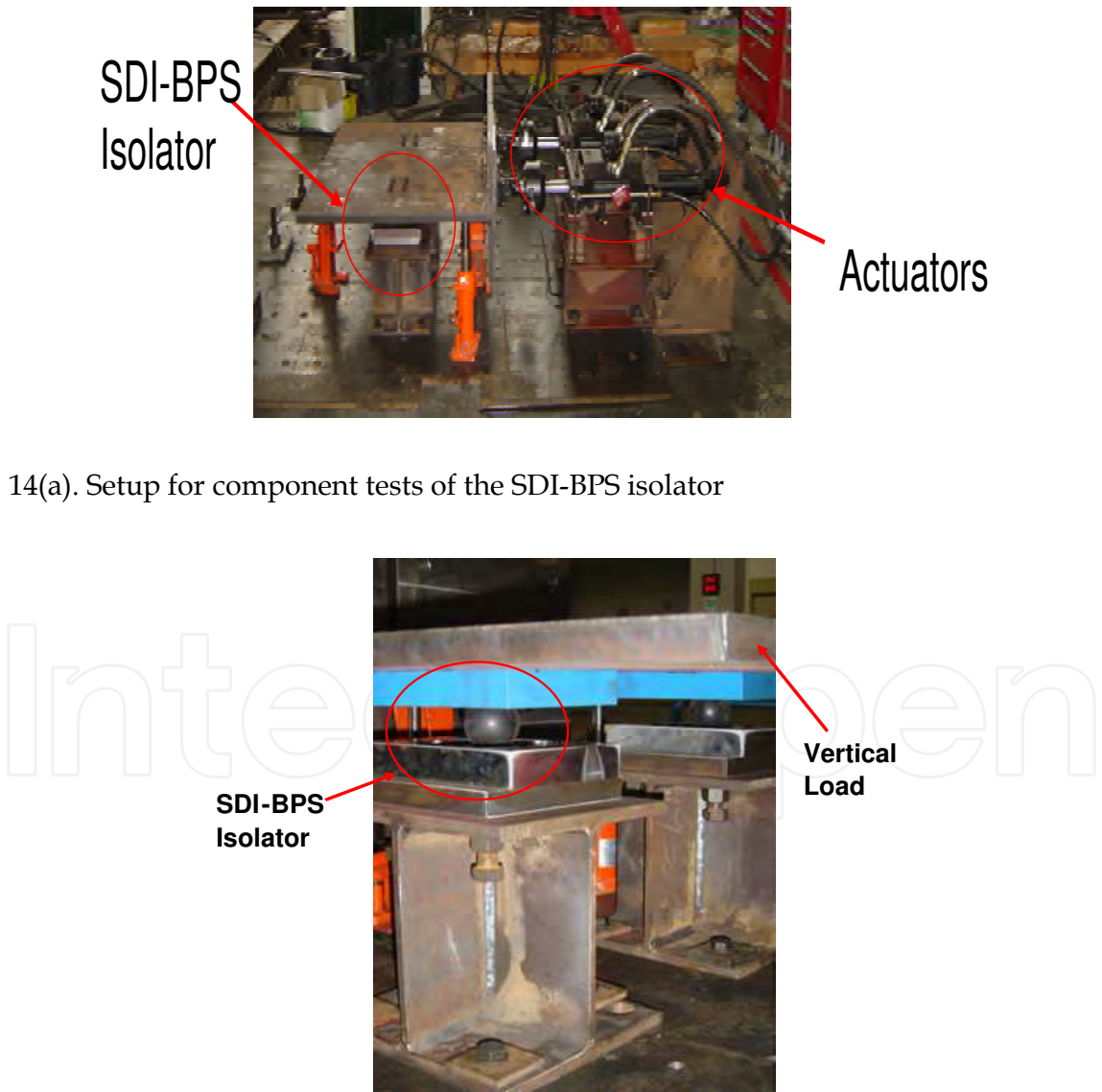
Fig. 14(b). Close view of component test of SDI-BPS isolator
