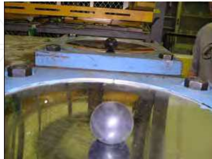
Fig. 3(a). Open-up view of ball pendulum isolation system
