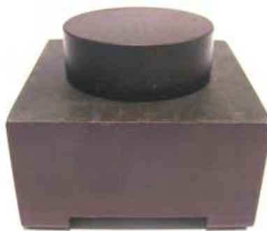
Fig. 21(a). Assembly of articulated slider coated with Teflon composite
