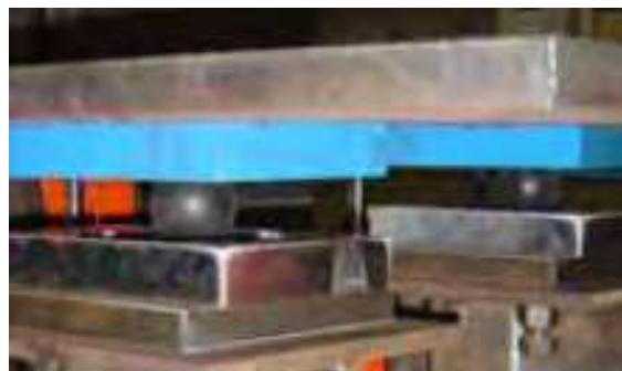
Fig. 3(b). Test set-up for ball pendulum isolation system
