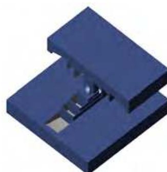
Fig. 10(b). Perspective view of multiple trench friction pendulum system
