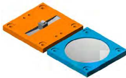
Fig. 11(a). Open-up view of first type direction optimized-friction pendulum system
