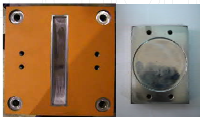
Fig. 20(b). An open-up view of the DO-FPS isolator with trench and concave surface
