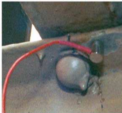
Fig. 2. AE Sensor on Brooklyn Bridge Floor Beam
