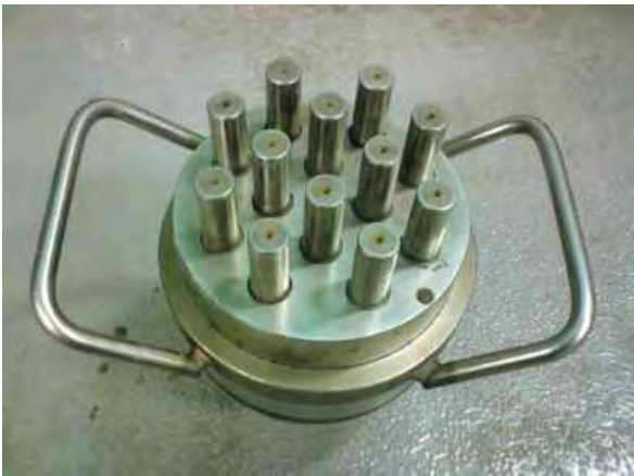
(b) Step 2: To set up the pestle into the mold
