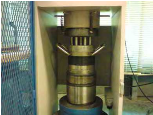
(c) Step 3: To press and form the recycling aggregates
