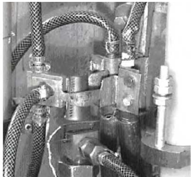
Fig. 22. Thermocyclic tests of the turbine blades with a thermal-barrier ceramic coating
