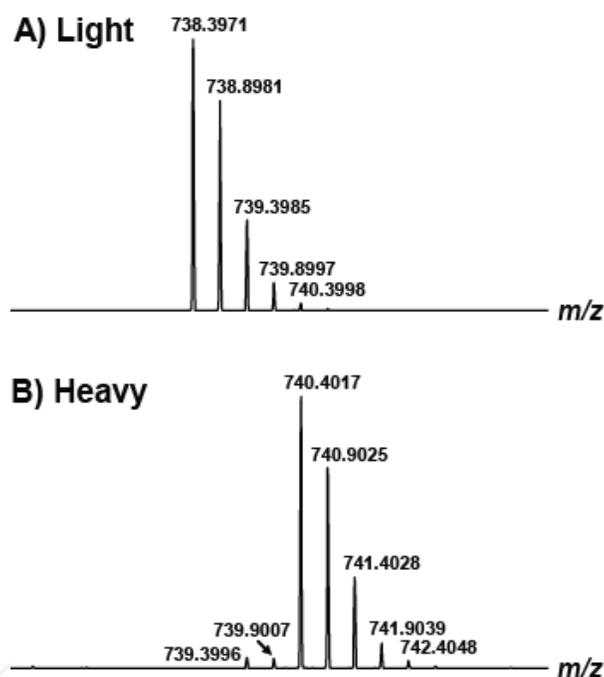
Fig. 5. Doubly charged tryptic peptide FLEQQNQVLQTK A) in the absence of  $^{18}O$  label and B) after incorporation of the label. The two-step labeling reaction in the presence of immobilized trypsin as described here ultimately results in the complete incorporation of two  $^{18}O$  labels, with no intermediary products present. The peptide isotope peaks in B) at  $m/z$  739.39 and 739.90 are due to impurities of commercial  $H_2^{18}O$ , containing only 97%  $^{18}O$ .
