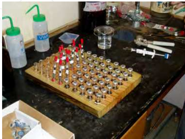
Fig. 2a. Charcoal filters replaced periodically. Fig. 2b. Charcoal filter extracted into vials.
