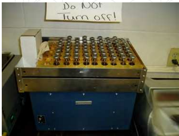
Fig. 3a. Vials shaken to extract MITC.
