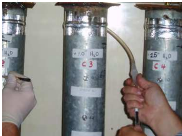
Fig. 2a. Charcoal filters replaced periodically. Fig. 2b. Charcoal filter extracted into vials.
