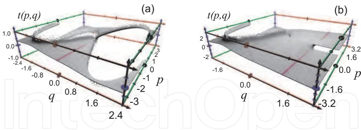
Fig. 4. Time values  $t(z)$  for the nonlinear oscillator with  $a = 1$ ,  $l = 2$ , and  $k = 9.8$ . (a)  $X = 0$  and (b)  $X = 1.5$ . The points coloured in cyan indicate the zero time points. Dimensionless units.
