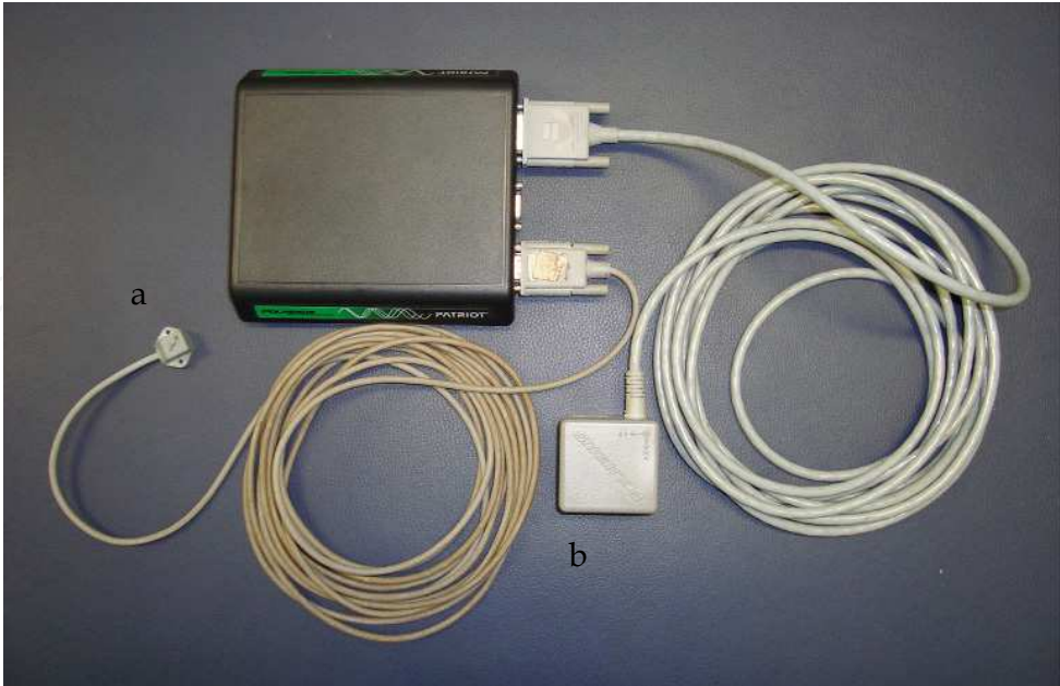
Fig. 1. Illustration of the Polhemus system. a) sensor coil; b) transmitting coil.
