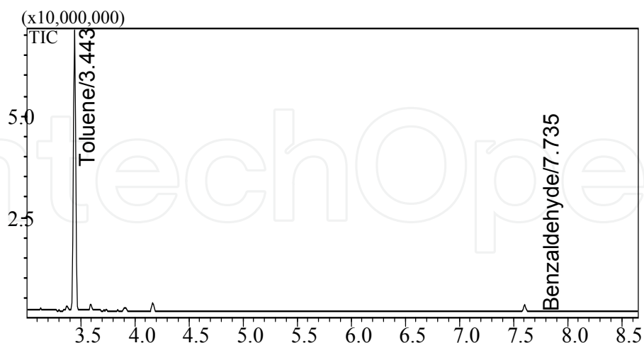
Fig. 4. A GC-MS spectrum of toluene/air mixture after EB-irradiation (inlet concentration of toluene was 151.9 ppm, dose was 53.6 kGy).
