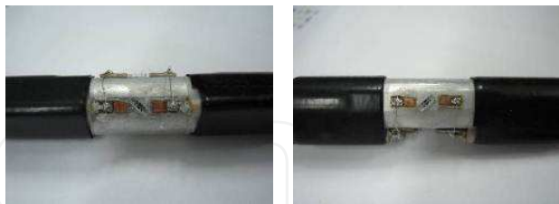
Fig. 35. The rotational shaft equipped with two SAWRs.
