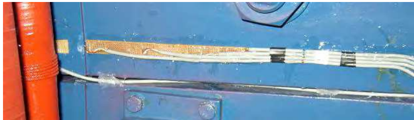
Fig. 6. Built-in Hall probes
