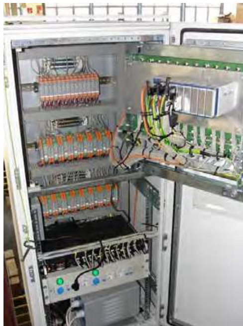
Fig. 16. Measurement cabinet with NIcDAQ9188 data acquisition system
