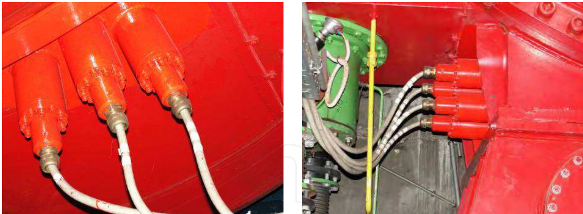
Fig. 15. Signal cable glands
