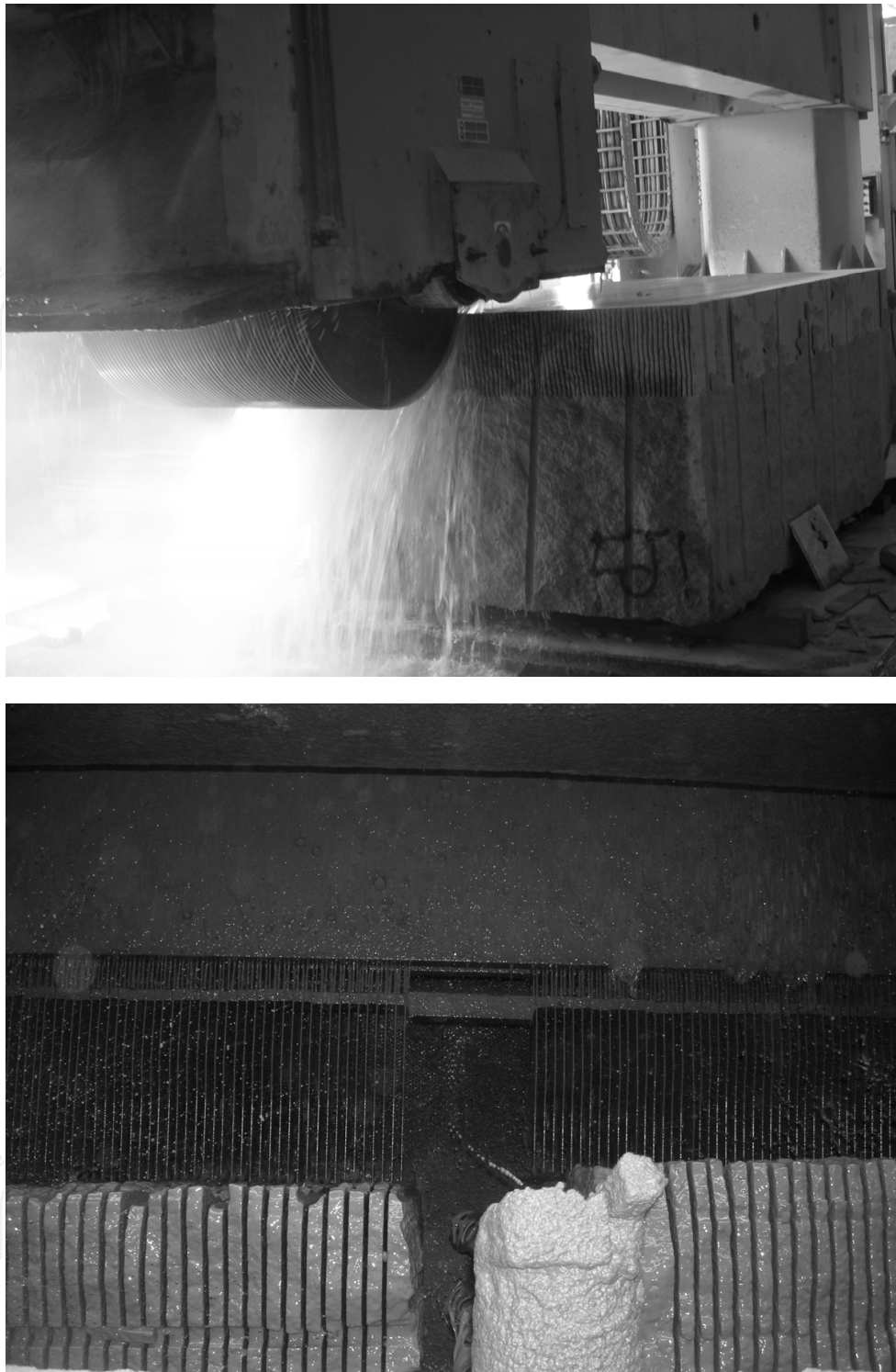
Fig. 1. Sawing operation of granite blocks.
