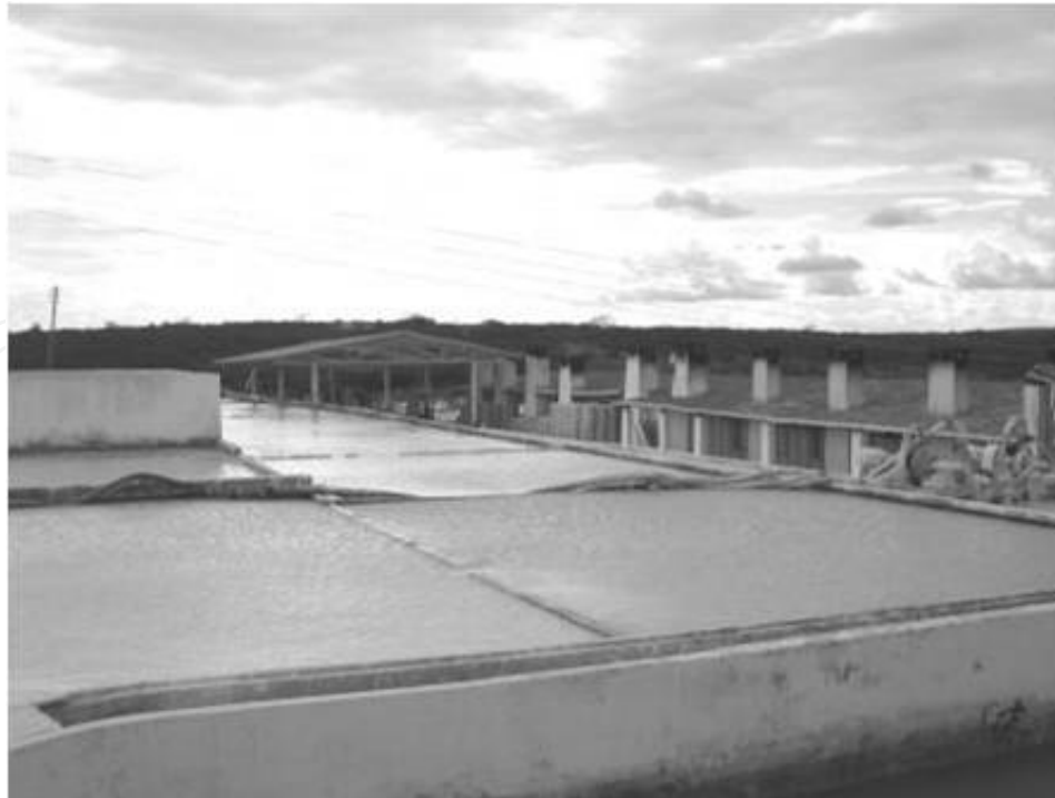
Fig. 8. Sedimentation tank used in the second step of kaolin processing
