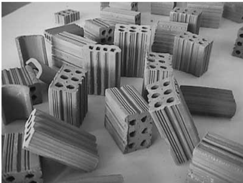
Fig. 4. Ceramic bodies containing granite sawing waste
