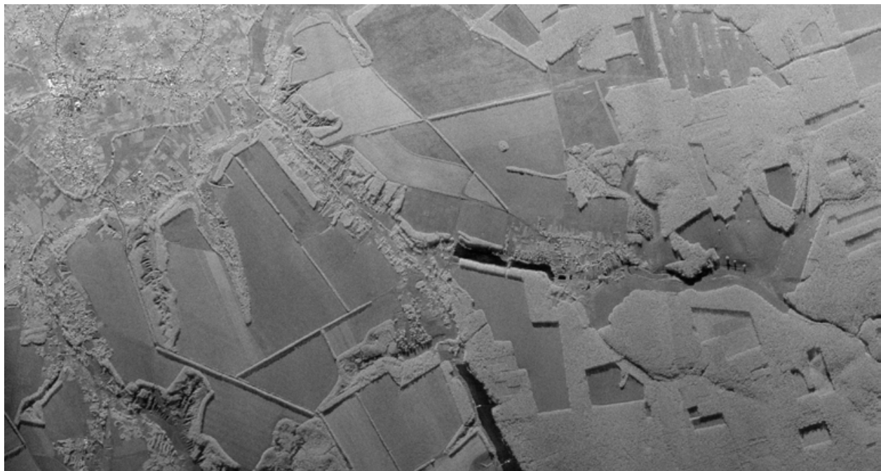
Fig. 17. An example of a 7-look SAR image obtained with the X-band SAR system.
