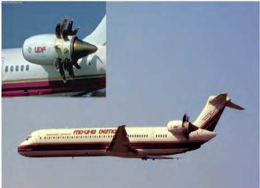
Fig. 20. GE36 Turbo-Prop demonstrator engine on MD-81 aircraft [21].
