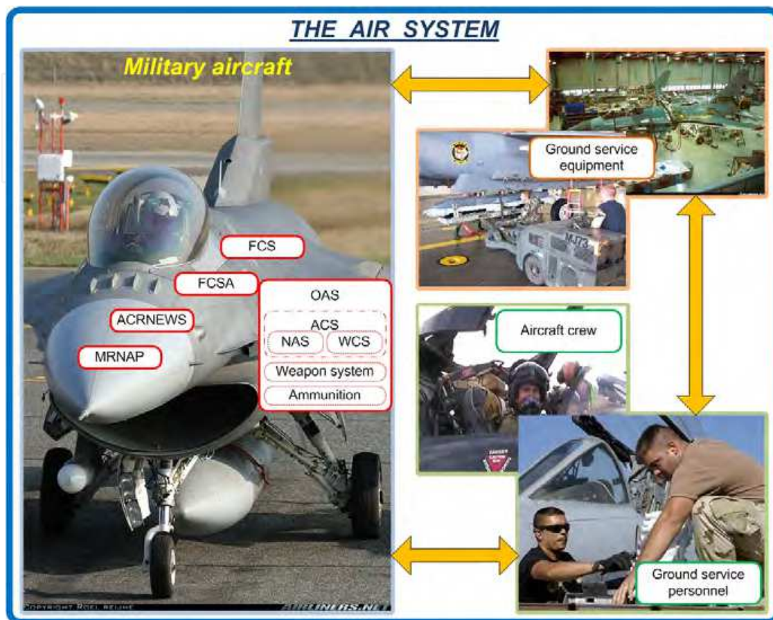
Fig. 1. Structural diagram of the military aircraft and the air system: FCSA – Flight Control System Actuators (frame construction with plating); FCS – Flight Control System; ACRNEWS – Airborne Communication, Radio Navigation and Electronic Warfare Systems.; MRNAP – Multifunctional Radar and Navigation and Aiming Pod; OAS – On-board Armament System; ACS – Armament Control System; WCS – Weapon Control System; NAS – Navigation and Aiming System.
