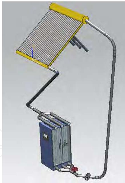
Fig. 24. Solar drying machine system
