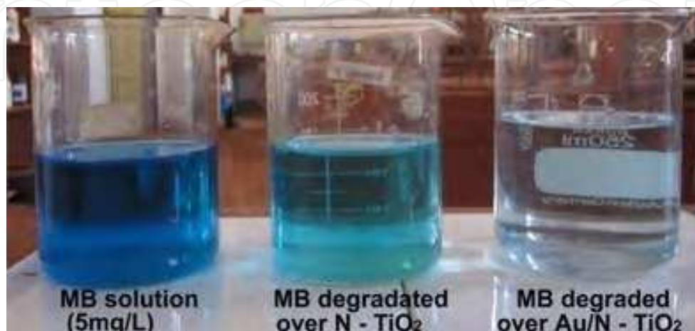
Fig. 1. Degraded methylene blue solution under 1 h exposure to sun light over N doped \text{TiO}_2 and Au loaded N doped \text{TiO}_2
