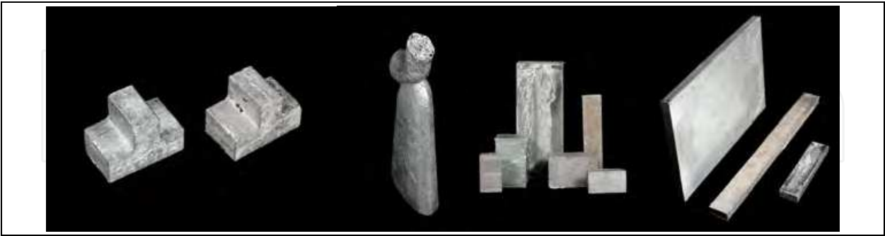
Fig. 14. 3D-parts of Al-alloy foams.
