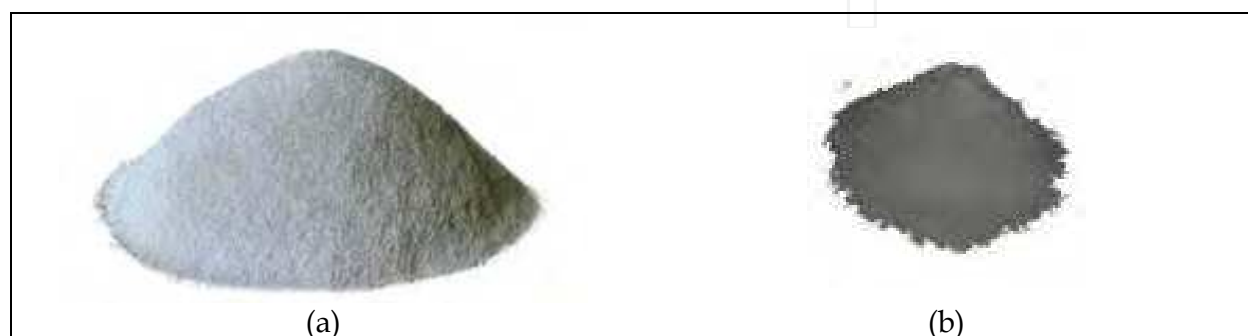
Fig. 3. Al-alloy and \text{TiH}_2 powders used in PM method.
