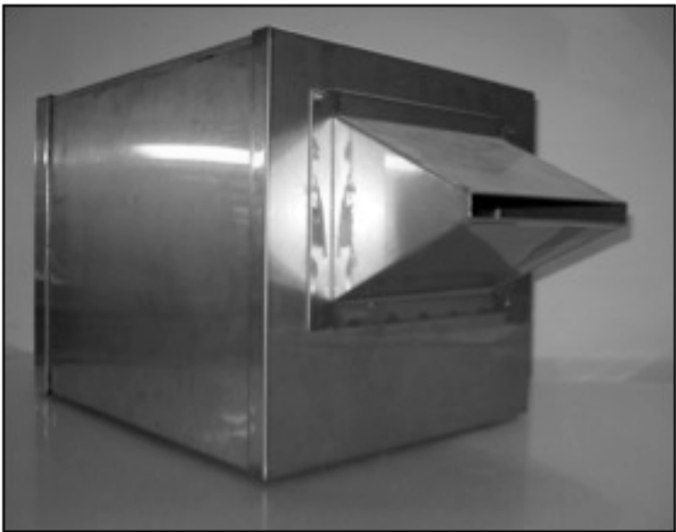
Fig. 1. Excito-repellency test chamber showing side of exit portal (Roberts et al., 1997).
