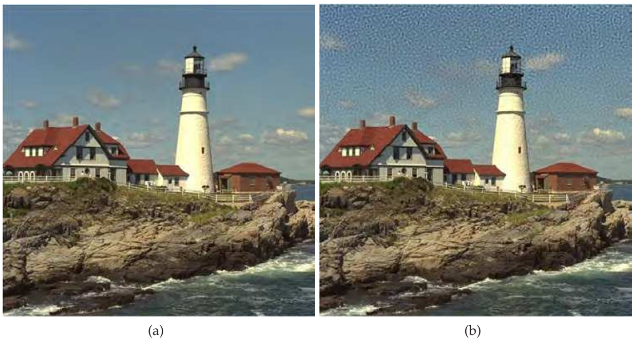
Fig. 1. Human vision system and images with identical PSNRs (Winker & Mohandas, 2008).
