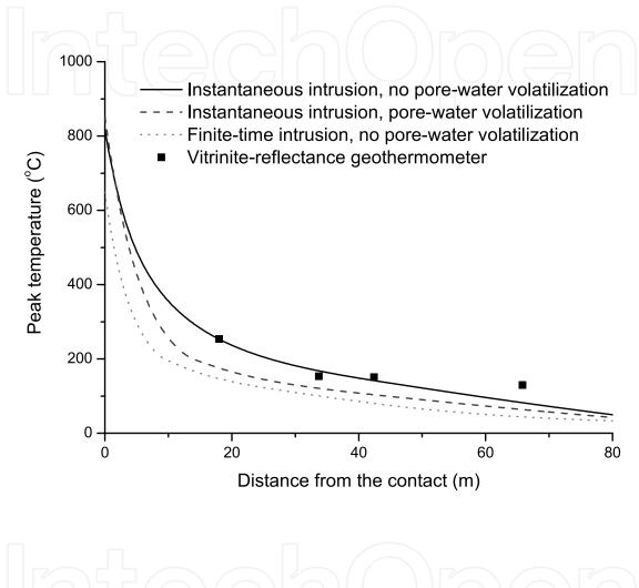
Fig. 2. Comparison between virtrinite-reflectance geothermometer of Baker et al. (1998) and peak temperature of host rocks predicted by three types of heat conduction models, assuming different intrusion mechanisms of magma and the state of pore water during cooling of magma
