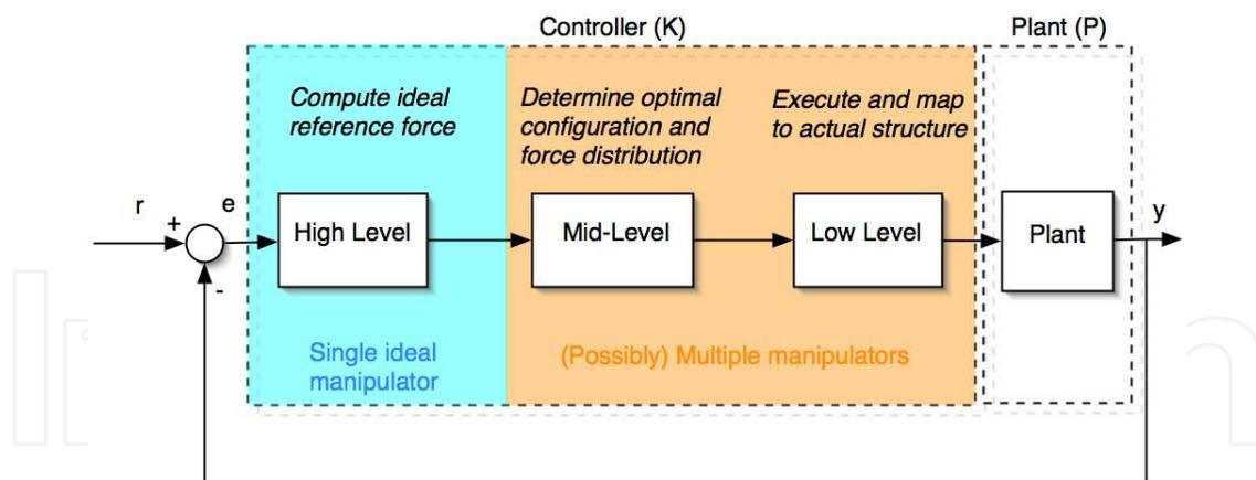
Fig. 5. Block diagram of hierarchical control scheme. This approach breaks a single complex problem into several smaller and more tractable problems.
