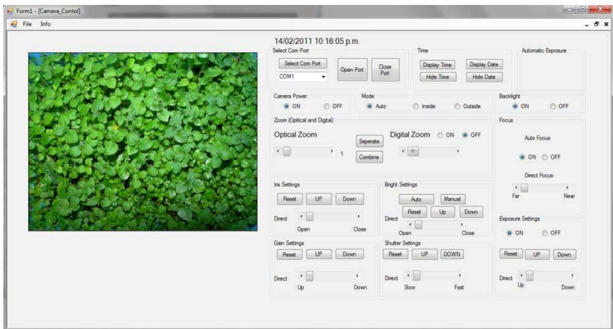
Fig. 12. User interface of the camera control program
