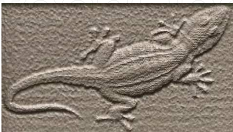
Fig. 22. AWJ-etched lizard on aluminum substrate (Webers et al., 2010)
