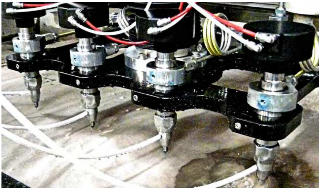
Fig. 25. Four nozzles mounted on a platform for increased productivity (Liu et al., 2011b)
