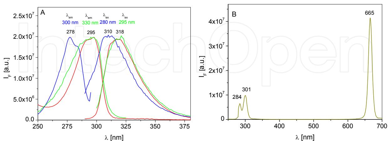
Fig. 4. (A) Excitation spectra ( $\lambda_{em}=300$  and 330 nm) and emission spectra ( $\lambda_{ex}=280$  and 295 nm) of extra virgin olive oil (green and blue) and tocopherol (red); the respective excitation and emission wavelengths are shown in the picture; (B) synchronous fluorescence spectrum ( $\Delta\lambda = 10$  nm) of extra virgin olive oil, (Sikorska et al., 2011).
