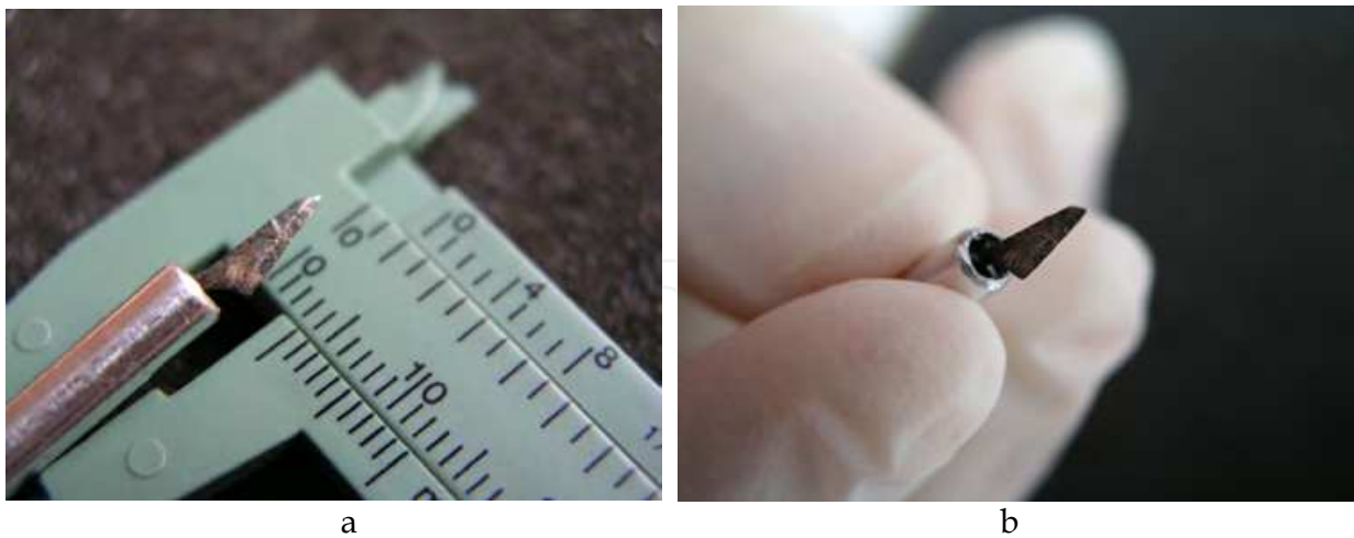
Fig. 6. Final prototype has an outer diameter of 4 mm
