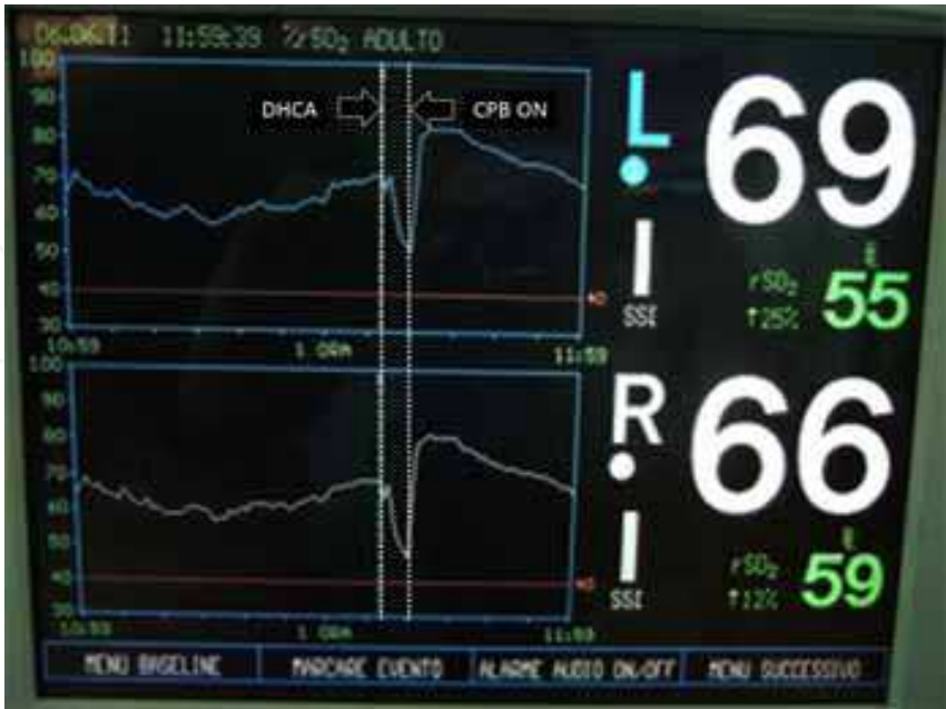
Fig. 5. Near infrared spectroscopy. (DHCA Deep Hypothermic Circulatory Arrest; CPB, cardiopulmonary bypass).
