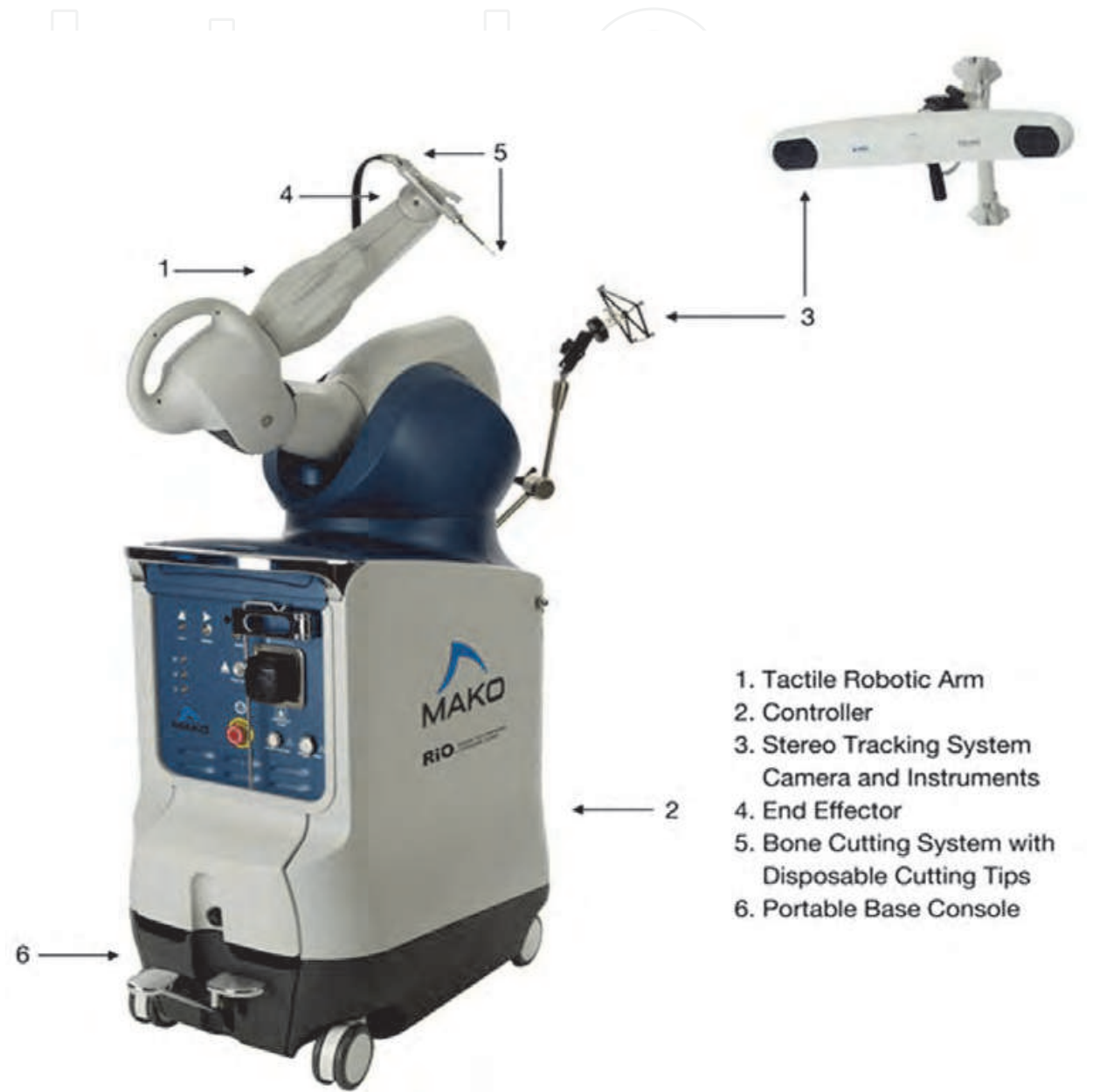
Fig. 10. MAKO Tactile Guidance System (TGS) (MAKO Surgical Corp., Fort Lauderdale, Fla)
