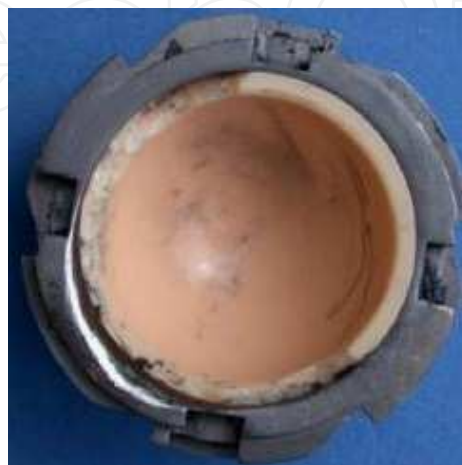
Fig. 10. Acetabular liner showing gross damage to the liner
