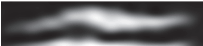
Fig. 9. Low-frequency illumination distribution of a typical bright and dark moiré fringes.
